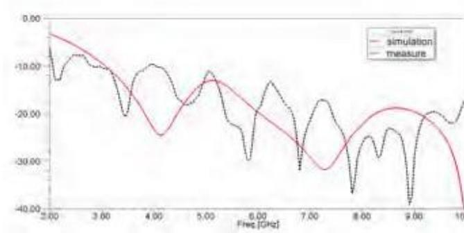
**Figure 3:** Measured and simulated diagrams the return loss of the proposed antenna
