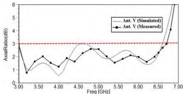
**Figure 5:** Measured and simulated diagrams the axial ratio of the proposed antenna.
