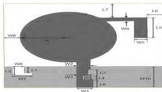
**Figure 2:** Geometry of the proposed CP square monopole antenna  $R = 6$ ,  $W_1 = 2$ ,  $L_1 = 1.5$ ,  $W_2 = 1.7$ ,  $L_2 = 2$ ,  $W_3 = 1.4$ ,  $L_3 = 1.5$ ,  $W_4 = 1$ ,  $L_4 = 1$ ,  $W_5 = 1.6$ ,  $L_5 = 4.8$ ,  $W_6 = 1.5$ ,  $L_6 = 2.2$ ,  $W_7 = 2.5$ ,  $L_7 = 3.4$ ,  $W_8 = 2$ ,  $L_8 = 1.8$ ,  $W_9 = 0.8$ ,  $W_{10} = 5$  (unit: millimeters).
