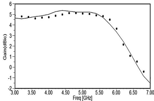
**Figure 4:** Measured and simulated antenna gains in the +Z-direction
